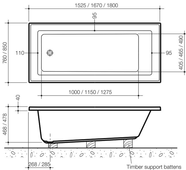
On the indicator lines, position and fix timber supports to base of the bath and floor with an approved floor and wall panelling adhesive or equivalent adhesive to provide a neat fit support. Ensure the rim of the bath is levelled during this procedure.
