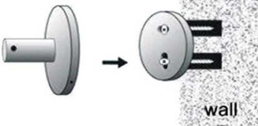
4. Put the base of bathroom accessory cover on the fixing blocks.
