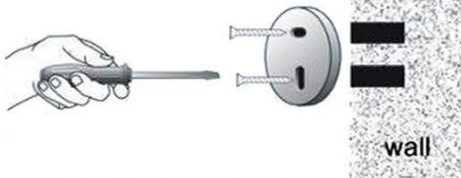
3. Put fixing block cover on the holes and fix firmly by expansion screws.
