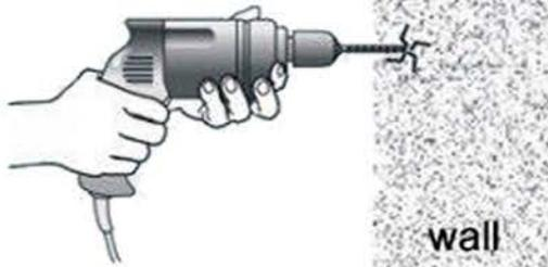
1. Put the fixing blocks (piece) over on the right place on the wall , and stay level, use marking pen through the holes of fixing block to mark out fixing spots on the wall. Then drill holes by electric hand drill with 6mm drilling bit on the spots.
