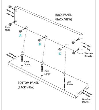
• Line up Back Panel Cam Nuts and Bottom Panel Cam Screws (A, B and C), push into position (see photo).
