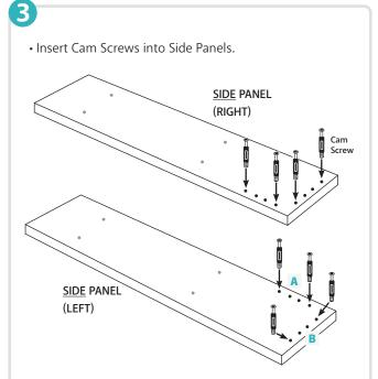
• Line up remaining holes (A and B) with Wooden Dowels in undershelf, and push into position.
