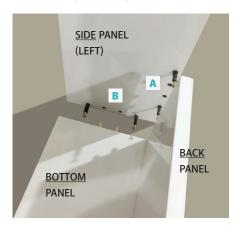
• On the Back and Bottom Panels, use a screwdriver to turn each Cam Nut until it locks into place. (If using an electric screwdriver be careful not to over-tighten as this may cause damage)
