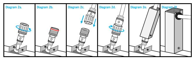
**Test A:** Ensure you connection is pushed in fully and screw cap is screwed on tightly with the arrows matching up. Once checked, tick this on page 11.
