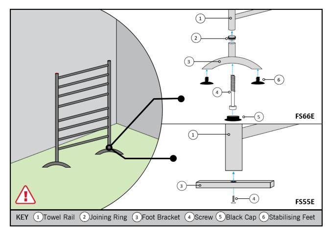
The Thermorail Free Standing models in this guide can only be installed with exposed wiring and is designed to be a portable unit and plug into a power point.
