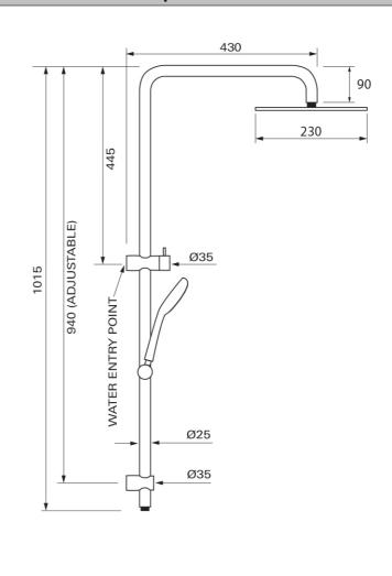
Note: All dimensions are in millimetres and are subject to normal manufacturing variations. Always use the physical product measurements for cut-outs and rough-ins as the technical details shown may differ from the actual product. Use acetic cured silicone sealant. Do not use epoxy type adhesives. Clean with damp cloth. Do not use abrasive cleaners, liquids or pastes.
