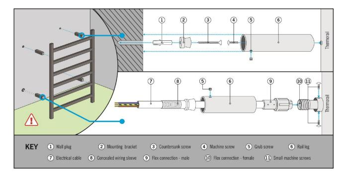
The Thermorail models in this guide can be installed with either concealed or exposed wiring, with the electrical supply connected at the bottom or top, left or right hand mounting point. This section concentrates on the concealed wiring method. For exposed wiring see page 6.
