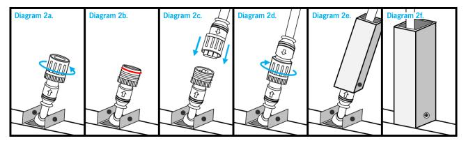
**Test A:** Ensure you connection is pushed in fully and screw cap is screwed on tightly with the arrows matching up. Once checked tick this on page 11.
