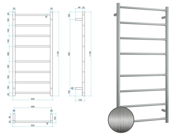
This rail has Multiflex wiring which means that there is a connection point on both the left and right hand side of the rail and the lead can be connected to either side. Being a dry electric element rail, this can be mounted either way up meaning the wiring can be from any of the four mounting points.
