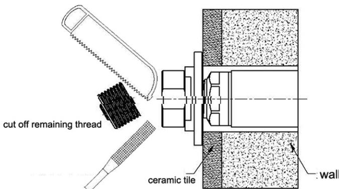
1. cut off remaining thread against to the cut off gauge.
