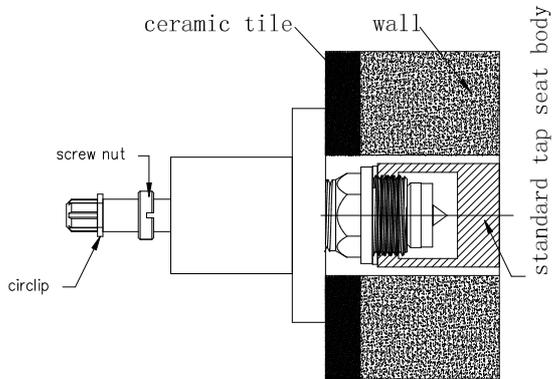
1. Put screw onto the stick of slow-opening valve.
