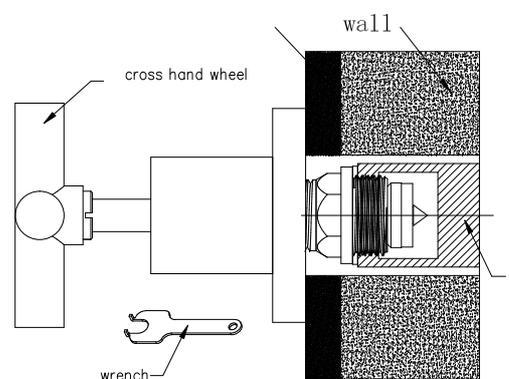
1. Put cross hand wheel onto stick of slow-opening valve, then adjust the rotation angle of hand wheel.
