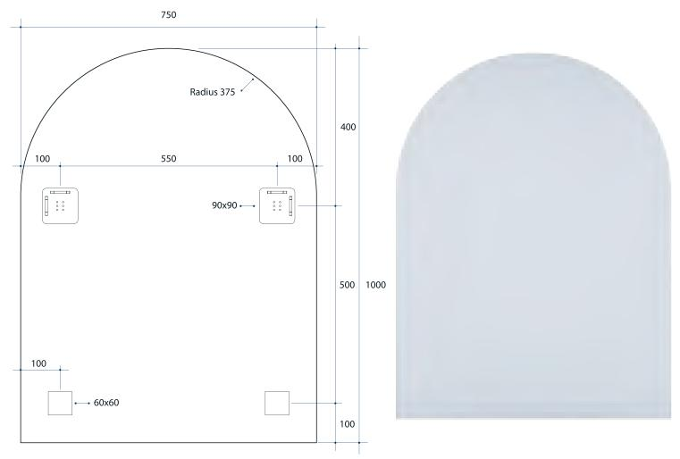
Note: All dimensions are in millimetres (mm)
