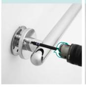
10. Rotate the flange cover so the hole is positioned over a new screw fixing point.
