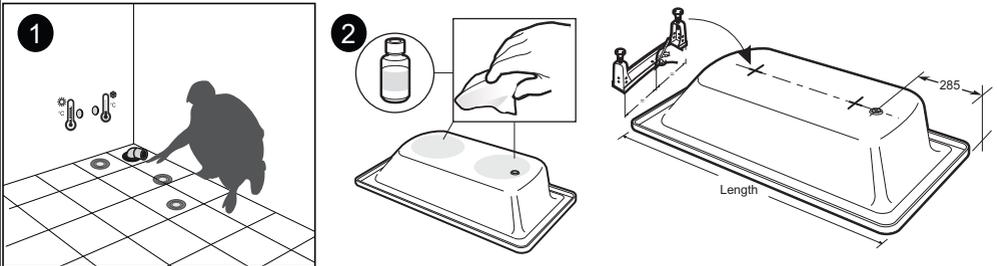
1. Before installation set out the pipe work for the bath and ensure it is aligned with the waste.
