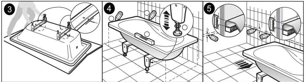
4. Place in position and use the adjusting screws to ensure the bath is completely level. Make sure that the underside of the bath is clear of any obstructions.
