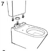
7.Place rubber seal into pan recess (DO NOT USE SEALANT). Place cistern screws into holes on the inside of cistern, making sure washers are located correctly. Gently lower cistern onto pan locating fixing screws into matching pan screw holes. Secure cistern to pan. Before tightened fully make sure cistern sits square and straight to pan.
