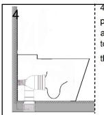
4.Align and push fully assembled toilet back to the wall
