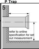
5.Set up waste pipe so that the end of the pan collar extends far enough from the finished wall to seal
