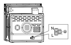
Disconnection from the supply may be achieved by having the plug accessible or by incorporating a switch in the fixed wiring in accordance with the wiring rules.
