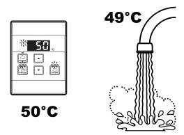
Depending on the weather conditions and the length of the pipe between the hot water unit and the outlet in use, there may be a variation between the temperatures displayed at the water controller(s) and the temperature of the water at the outlet.
