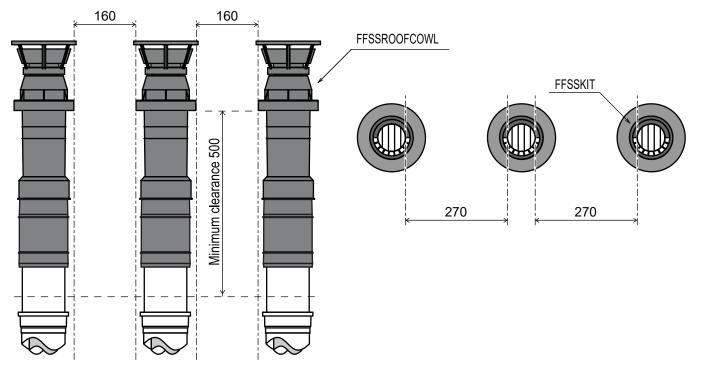
The terminal clearances stated in AS/NZS 5601 do not apply to the Rinnai internal gas continuous flow water heaters when they are installed side by side.
