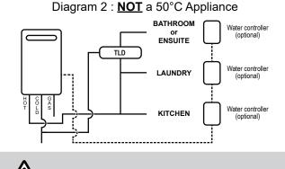
Universal water controllers are available as an optional extra and will function as described in the Operation Section of this manual. Refer to "Water Controllers Limitations" on page 24 to confirm the maximum number and combination of water controllers that can be fitted.
