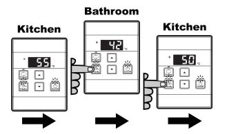
As a safety precaution, if a Kitchen Water Controller's temperature is set above 50°C, transferring and then returning 'priority' to the Kitchen Water Controller will result in a default set temperature of 50°C being selected. This is a safety feature.
