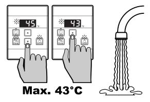
Whilst hot water outlets are open the set temperature may be lowered. However they cannot then be raised above 43°C. In addition transfer of 'priority' between controllers is not possible. These are safety features.
