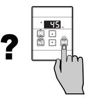
There is no need to turn the water controller(s) off after use. However, if you prefer to turn the water controller(s) off, your selected temperatures to a maximum of 50°C will be stored in the system memory at all times whilst mains power remains connected.
