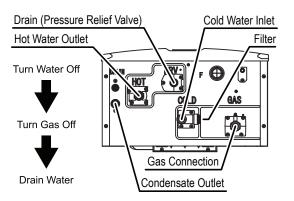
If freezing conditions are expected, turn off water and gas, and drain all water from the appliance. If power and the automatic frost protection are connected, freezing will be prevented. (Anti-frost protection is fitted as standard equipment on all hot water units).
