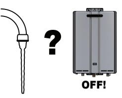
At low water flows, the hot water unit may extinguish without warning. Opening the tap further will restart the heating appliance.
