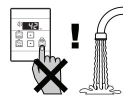
**DO NOT** push the On/Off button on any Water Controller when the water heater 'In Use' indicator is illuminated as this will turn off the water heater causing the water to go cold. Someone maybe in the middle of having a shower or filling a bath.
