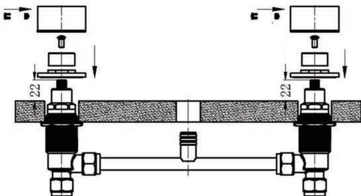
1. plug the assembled kit (picture 2) from the bottom side of the counter, and adjust the height as the picture.
