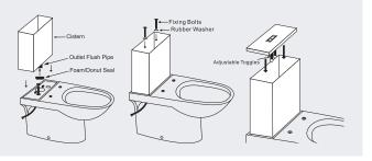
Before fixing the toilet to the floor, connect the water supply and ensure that the toilet is working correctly by doing several flush tests, checking for leaks. Once you are confident that there are no leaks and the toilet is working correctly install the Pan into the Floor Fixing Kit provided and apply a bead of Wet Area Silicone around the base of the Pan (you will need to allow for the recommended drying time). Install the side white cap over the side entry hole that was not used.
