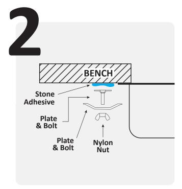
Plates & bolts should be positioned 10mm from the sink edge.
