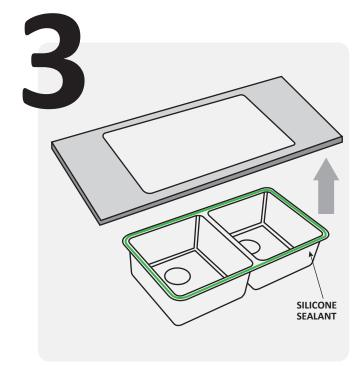
Clean the bottom of the countertop and the top flange (or lip) of the sink with methylated spirits. Then apply a bead of silicone to the top edge of the bowl.
