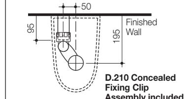
**D.210 Concealed Fixing Clip Assembly included with shroud**
