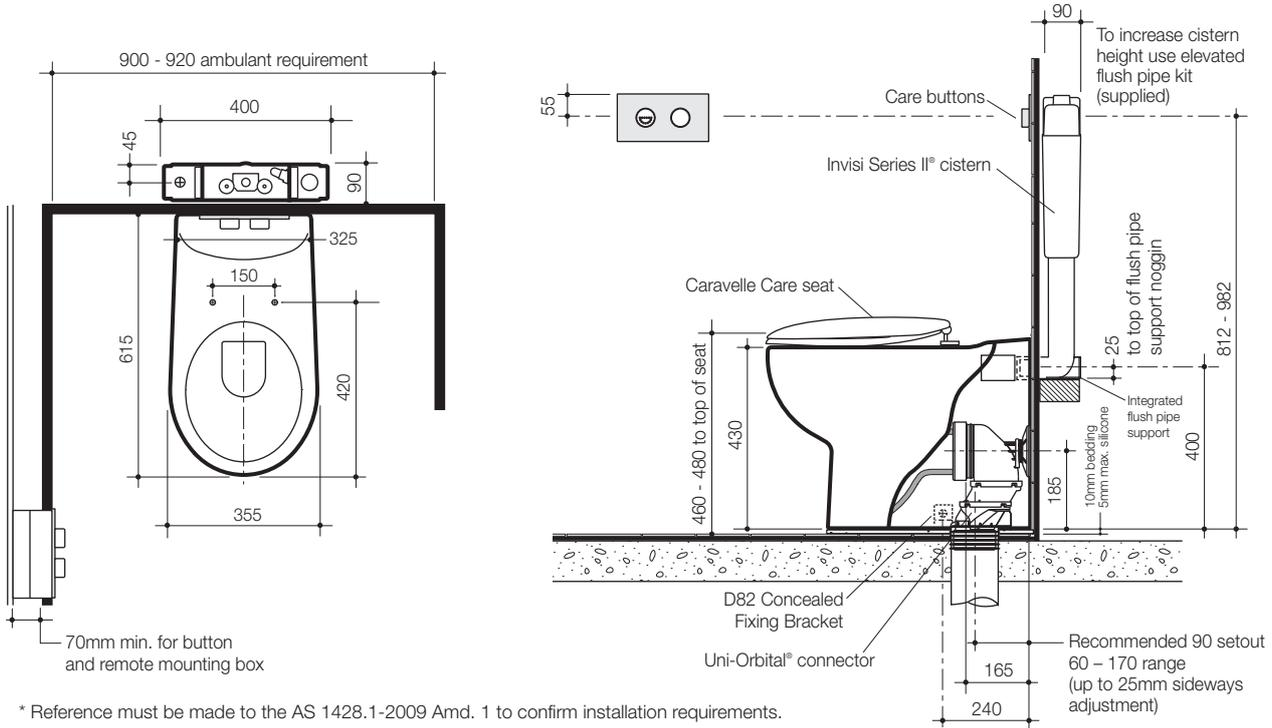
\* Reference must be made to the AS 1428.1-2009 Amd. 1 to confirm installation requirements.
