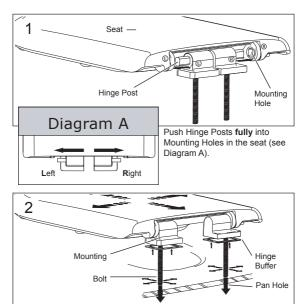
Ensure the Hinge Buffers are fitted to the underside of the Mountings. Lower seat onto pan, sliding bolts through pan holes, utilising the bolts X-Y adjustment to position the seat.
