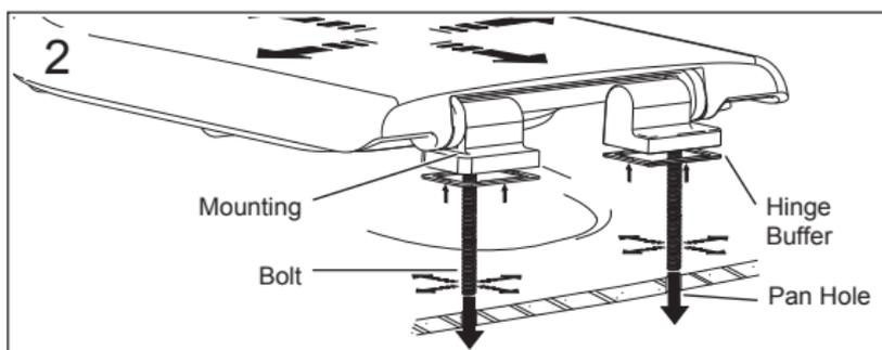
Ensure the Hinge Buffers are fitted to the underside of the Mountings. Lower seat onto pan, sliding bolts through pan holes, utilising the bolts X-Y adjustment to position the seat.
