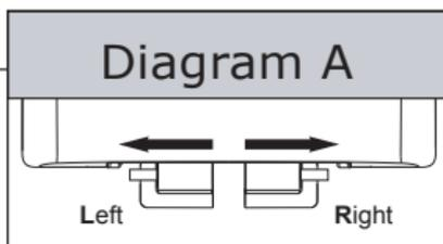
Push Hinge Posts **fully** into Mounting Holes in the seat (see Diagram A).
