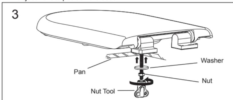
Check that the seat is correctly positioned on the pan. Slide Washer up to base of Pan and tighten Nut firmly using the Nut Tool.
