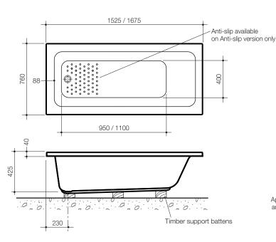
On the indicator lines, position and fix timber supports to base of the bath and floor with an approved floor and wall panelling adhesive or equivalent adhesive to provide a neat fit support. Ensure the rim of the bath is levelled during this procedure.
