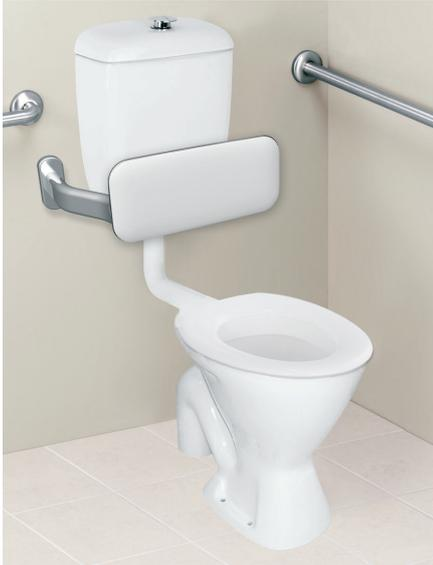
A pedestal type 6/3 litre dual flush **Care Pan** installation designed to provide a raised seat height of between 460-480mm for accessible applications . The versatility of the **Care Pan** makes it ideal for use by both the ambulant people with disabilities and wheel-chair users including wheeled commode chairs.
