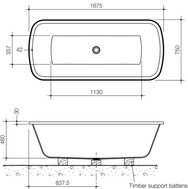
On the indicator lines, position and fix timber supports to base of the bath and floor with an approved floor and wall panelling adhesive or equivalent adhesive to provide a neat fit support. Ensure the rim of the bath is levelled during this procedure.
