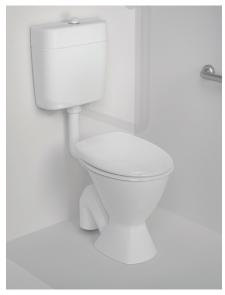
A pedestal type 4.5/3 litre dual flush Care 100 toilet suite installation designed to provide a raised seat height of between 460-480mm for accessible applications &. The versatility of the Care 100 suite makes it ideal for use by both the ambulant people with disabilities and wheel-chair users including wheeled commode chairs.
