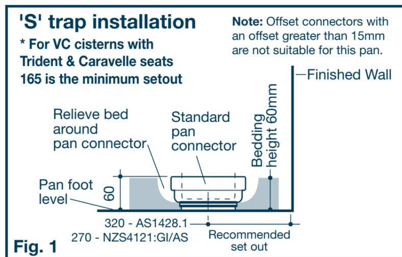
**IMPORTANT:** ALL DIMENSIONS ARE TO THE UNDERSIDE FOOT LEVEL OF THE PAN. IT IS IMPORTANT TO MAKE A HEIGHT ALLOWANCE FOR BEDDING.
