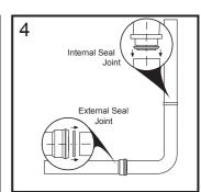
Assemble the Extended Mid Level Flushpipe (Refer to installation instruction in flushpipe)
