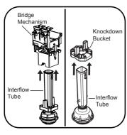
2a. Remove Outlet Valve from Bridge Mechanism by spreading the Flush Lever arms to clear the clips on the Interflow Tube.
