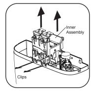
1. Pull both clips on front of cistern back to release Bridge mechanism. Remove inner assembly from the cistern by pulling upwards.
