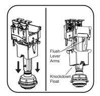
3. To reassemble the Outlet Valve, slide the Interflow Tube back through the Knockdown Float and clip into arms of the Flush Lever.
