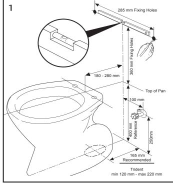
Check that the pan is installed within dimensional tolerances. Mark out the fixing holes for
