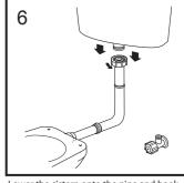
Lower the cistern onto the pipe and hook it over the mounting screws. Hand tighten the nut.
