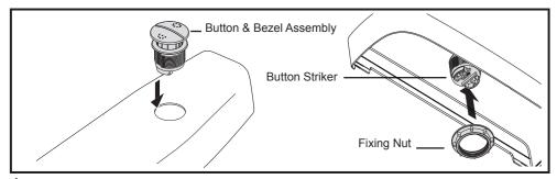
${f 1}$  . Insert button and bezel assembly into hole provided in cistern and fix in place using fixing nut. NOTE: The Half Flush Button must be on the left hand side.
