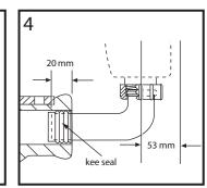
Cut the flush pipe to dimensions shown. Lubricate the kee seal with soan and water and fit the pipe into the pan. Fit the coupling nut and kingco onto the flush pipe
