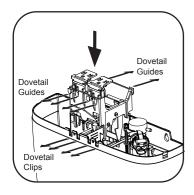
4. Slide inner assembly back into cistern ensuring the dovetail guides at the rear line up and the dovetail guides at the front clip into place.
