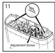
Actuate the inlet valve at least once to purge any trapped air in the valve Adjust the water level to the WL mark
