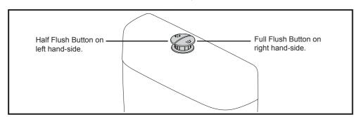
$oldsymbol{3}$ . Replace lid complete with button and bezel assembly and test both buttons to ensure they engage the platforms and activate the outlet valve.
