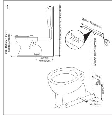
Check that the pan is installed within dimensional tolerances. Mark out the fixing holes for the cistern on the wall making sure they are level.
