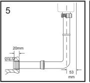
Cut the flushpipe to dimensions shown. Lubricate the kee seal with soap and water and fit the pipe.
