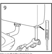
Make sure that the strainer is in place. Then fit the water supply pipe
