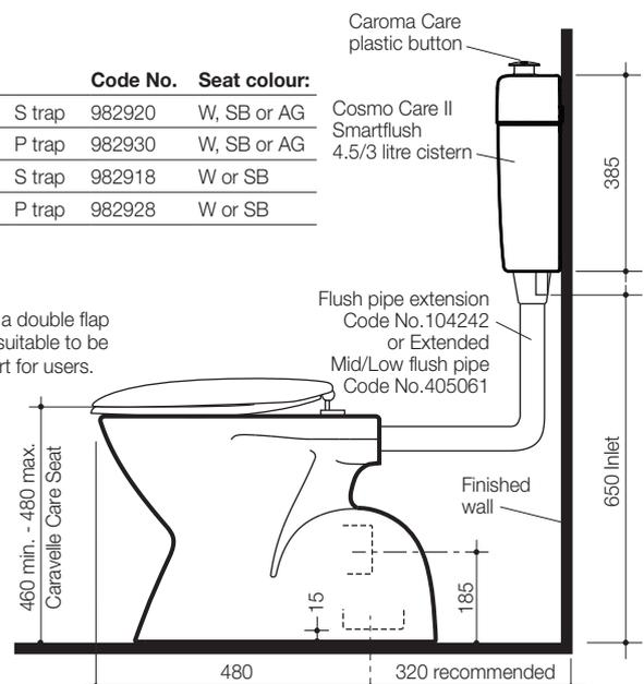
**Note:** The lid on a double flap toilet seat is not suitable to be used as a support for users.
