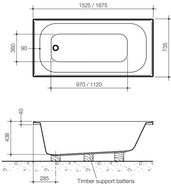
On the indicator lines, position and fix timber supports to base of the bath and floor with an approved floor and wall panelling adhesive or equivalent adhesive to provide a neat fit support. Ensure the rim of the bath is levelled during this procedure.
