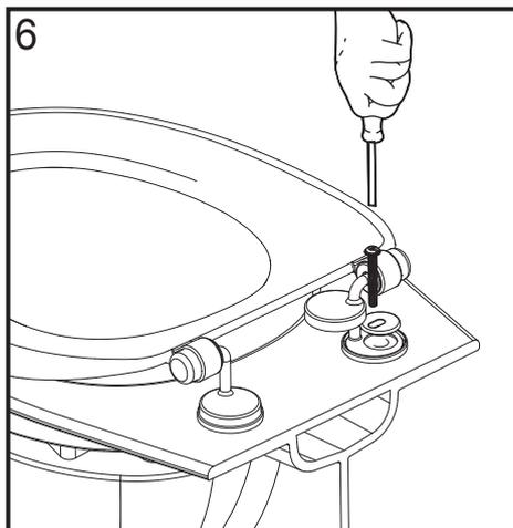
6 Remove the steel cover, insert the plastic washer and loosely bolt the hinges to the pan.
