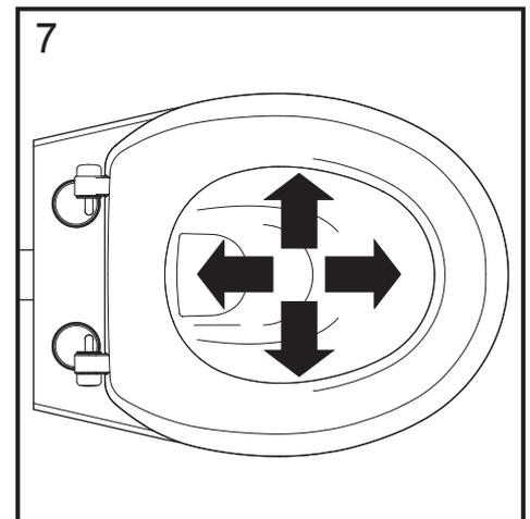
7 Position the Seat on the Pan then fully tighten the bolts, replace the steel cover and ensure seals are firmly in place at base of hinge posts
