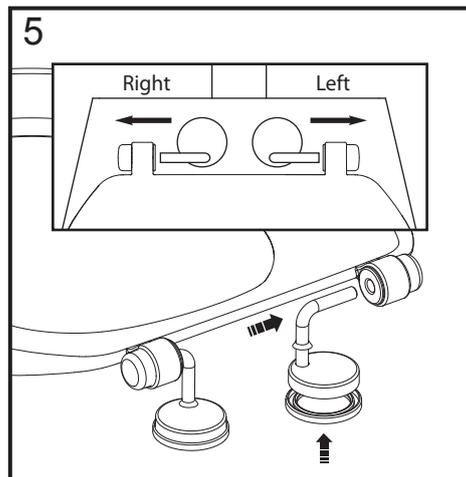
5 Insert the left hand and right hinges. Push on rubber pad to base of stainless steel hinge and rubber seal over hinge post.
