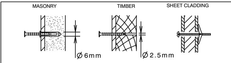
1. Use the screws and plugs for masonry, and screws only for timber. Butterfly Toggle (not supplied) should be used for sheet cladding.
