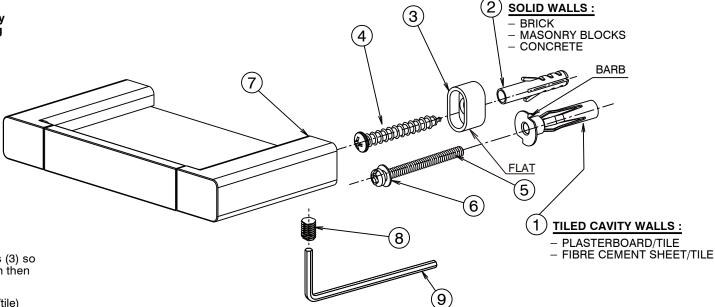
3) Install the shelf (7) onto the mounting brackets (3) Push the shelf against the wall surface while tightening the grub screws (8) using the 2.5mm allen key (9) provided. Ensure that the grub screws (8) engage with the flats on the mounting brackets (3) before tightening.
