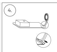
FIT GASKET TO SINK ENSURING DOUBLE THICKNESS AT THE CORNERS USING THE SEALING TAPE SUPPLIED.
