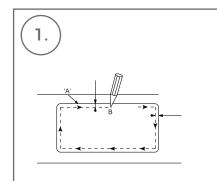
USING THE CUT OUT TEMPLATE PROVIDED, MARK THE CUT OUT LINE ON THE BENCHTOP
