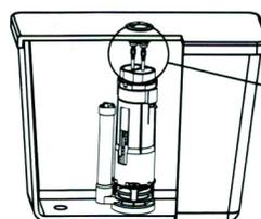
Button rods must be just clear of the valve pads
