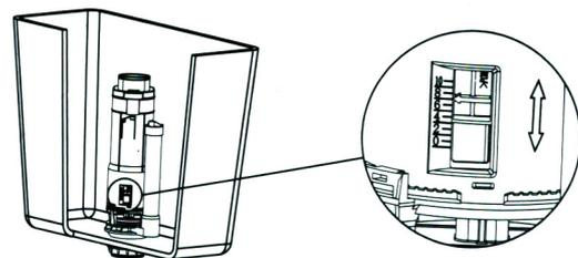
The full flush volume can be adjusted by changing the residual water level in the cistern. Move the adjuster DOWN to increase the volume. Move the adjuster UP to decrease the volume.
