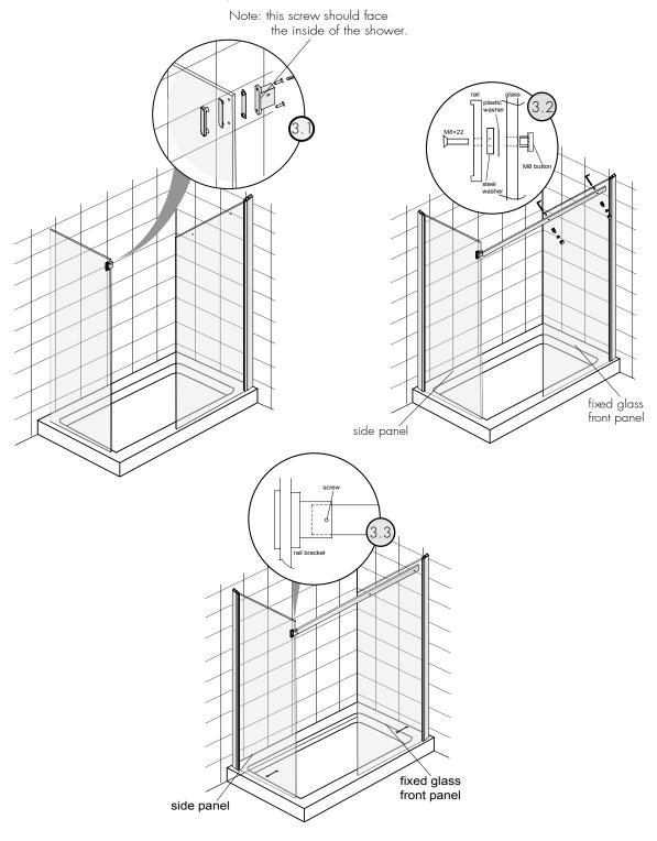
Ensure a plastic glass protector is used between all metal parts and the glass.
