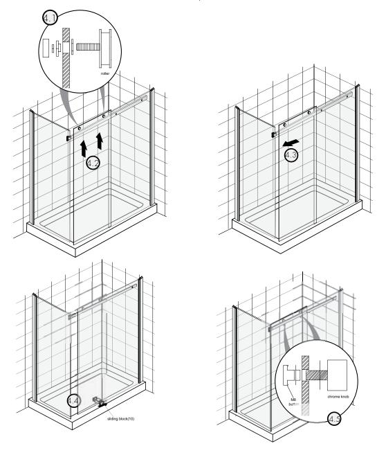
Ensure a plastic glass protector is used between all metal parts and the glass.
