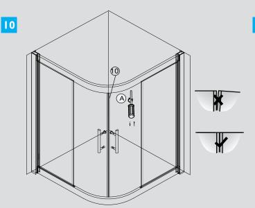
Adjust the sliding doors(4) using the screws located on the bottom of top roller assemblies(13). Adjust rollers so that the sliding doors (4) are parallel to the fixed panels(3) and parallel to each other. Note: Do not overtighten top rollers as this will cause the bottom rollers to jamb and or break.
