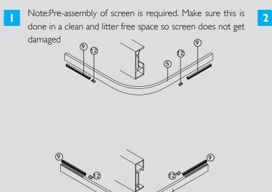
Insert fixed panel end block(12)first then short fixed panel seal(9)into slot on both bottom and top rails(5)(6). (Usually comes preinstalled in top and bottom rail.)
