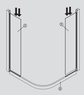
Push fixed panels(3) into seal that is located in the bottom rail(6).Make sure that the panel is firmly up against the fixed panel block(12)and fully inserted into the short seals(9). Hint-Wet the edge of glass &seal to make it easier to insert panel.
