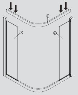
Push fixed panels(3) into seal that is located in the top rail(5). Make sure that the panel is firmly up against the fixed panel block(12)and fully inserted into the short seals(9). Hint-Wet the edge of glass and seal to make it easier to insert panel.
