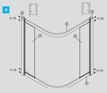
Screw the fixed panel extrusion(2) to the top and bottom rals. Please make sure that the location of the screw holes in the fixed panel extrusion line up with the holes in the top and bottom rails.
