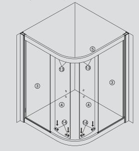
Adjust the sliding doors(4) using the screws located on the bottom of top roller assemblies(13). Adjust rollers so that the sliding doors (4) are parallel to the fixed panels(3) and parallel to each other. Note: Do not overtighten top rollers as this will cause the bottom rollers to jamb and or break.
