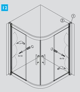
Drill 4 equally spaced holes on the inside of the screen.Fix off wall jambs(1) to the fixed panel extrusion(2) using the screws supplied. Cap all screws.
