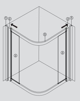
Adjust fixed panel extrusions(2) in or out on the wall jambs(1) so that the top rail(5) is horizontal and the whole screen sits square on the shower base/shower area.(B=C=D)
