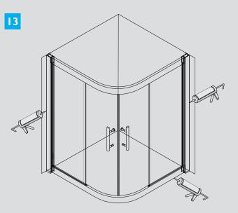
Apply silicone sealer around all external joints of shower screen and **allow 24 hours for silicone to set.** Do not silicone inside the shower screen.
