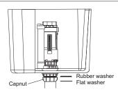
Capnut must be hand tightened to correctly seal flush pipe
