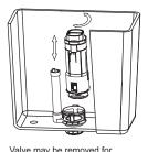
Valve may be removed for service - twist to unlock
