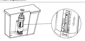
Half flush volume can be adjusted by moving the side float up or down. Moving the float DOWN increases the half flush Moving the float UP decreases the half flush
