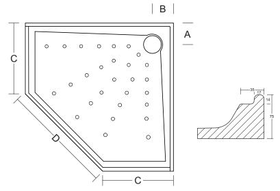
The Evo polymarble shower base is self-supporting eliminating the need for a mortar bed. It features an anti-skid surface and dome covered waste as standard.
