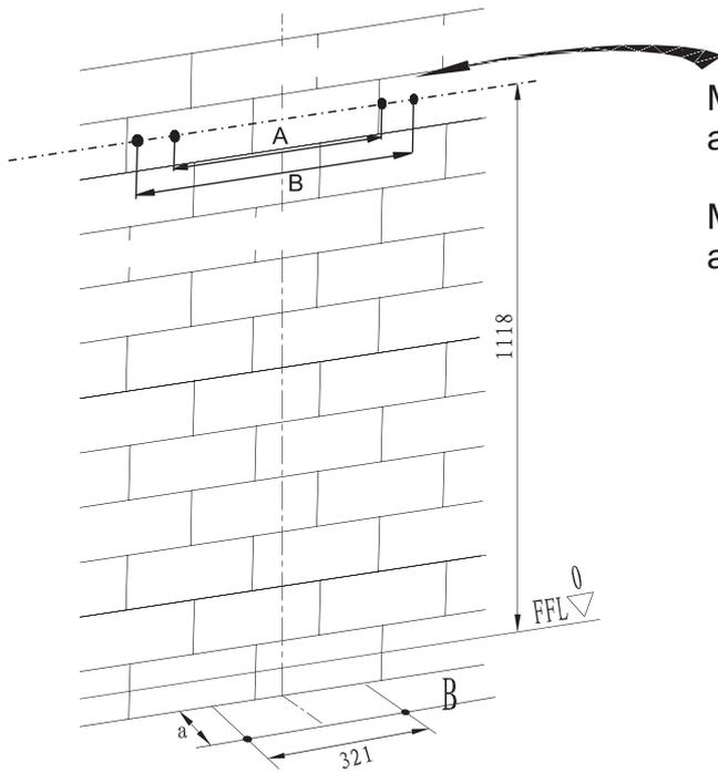
Measurement (A) = 497mm if the L brackets are to be installed facing inwards.
