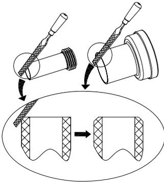
Clean and chamfer cut edge as shown
