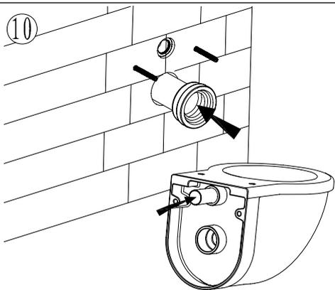
Insert the sewer pipe onto the wall connection and fit the flush pipe onto the VC inlet spigot
