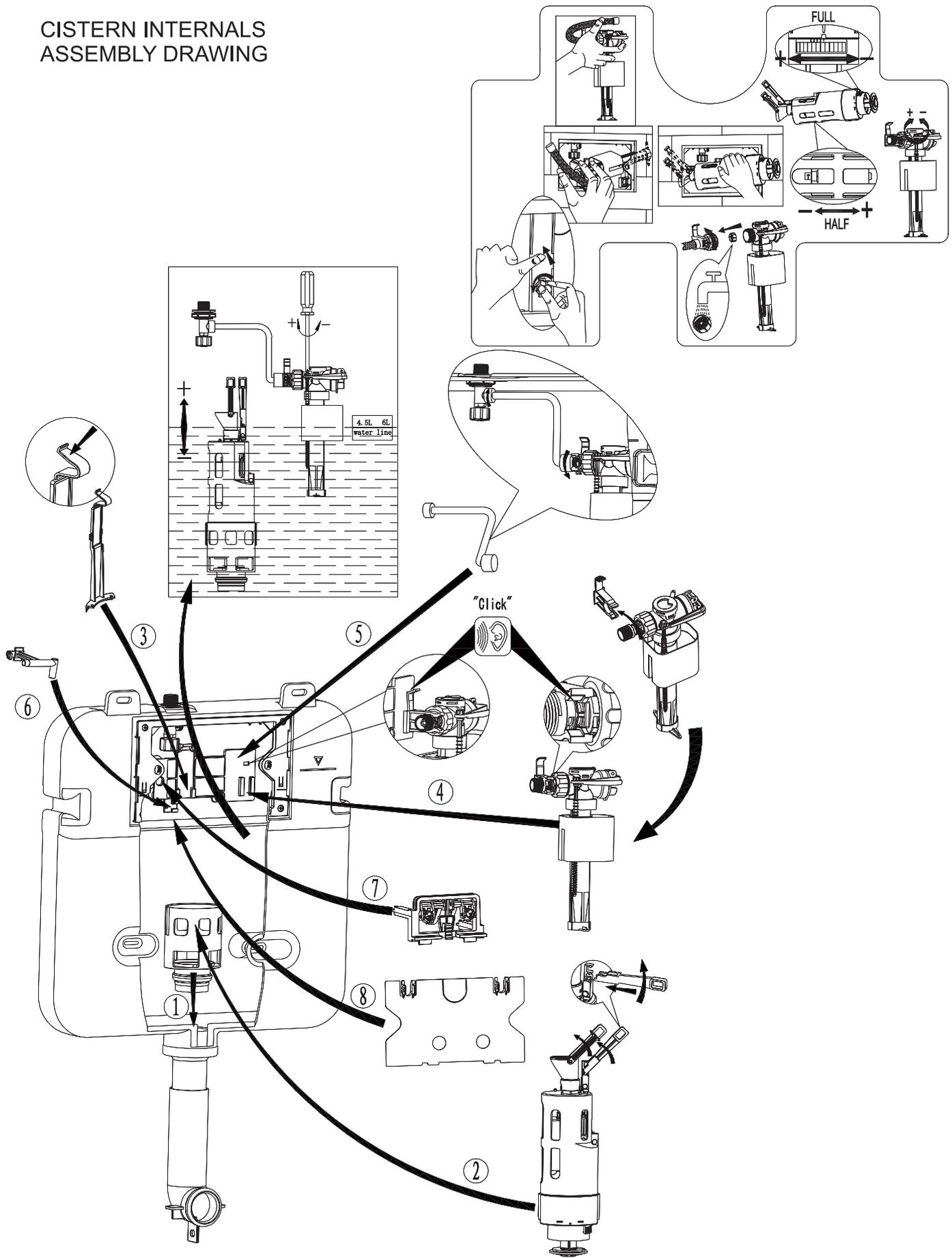
Above internal parts are all already installed in the tank and this diagram is for reference only
