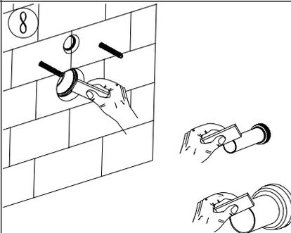
Apply lubricant to the cut pipe end
