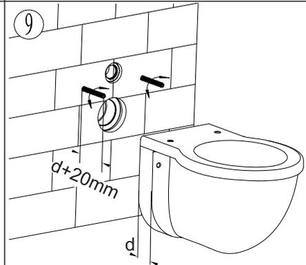
Adjust exposed pan bolt length to  $d+20\text{mm}$
