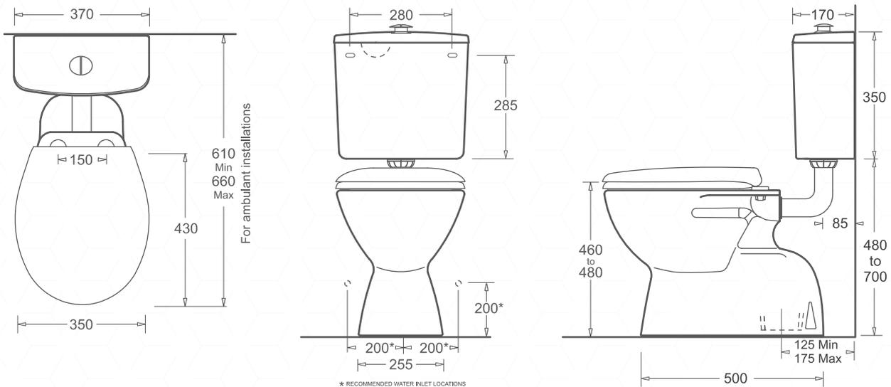
For Ambulant compliance the design of the installation space must comply with AS1428.1 - Design for access and mobility
