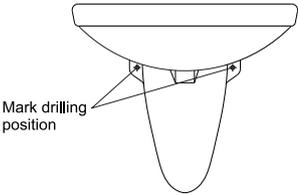
**2** Drill hole with 8Ømm drill bit.
