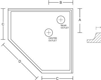
The Flinders Polymarble shower base is made from high strength polymarble compound - which is a hardwearing, solid, fully moulded material that is ideal for bathroom surfaces.
