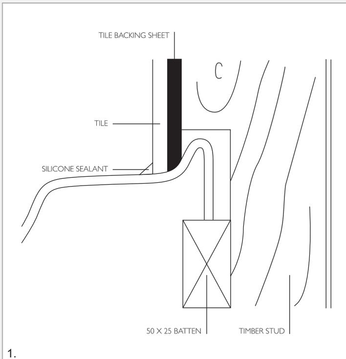
Check that your floor is level and secure. Your Marbletrend bath does not need to be supported by a mortar bed. To adhere your bath to the floor, simply run a generous bead of silicone along the timber support and allow sufficient time to cure. Timber supports must have full contact with floor to achieve correct support for bath.
