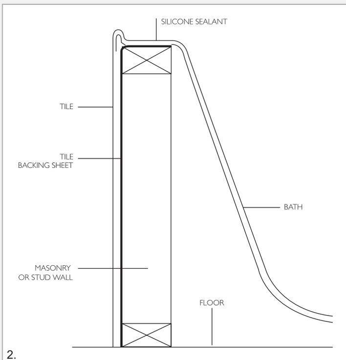
2. The front edge and sides of the bath are to be supported by a mini wall that can be constructed out of timber or masonry.
