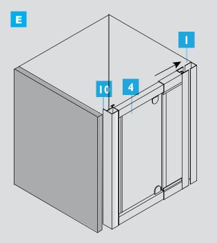
Slide front assembly (4) into jamb (1)
