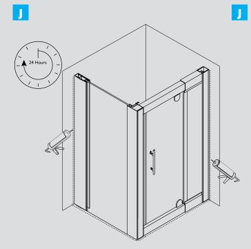
Apply silicone sealer around all external joints of shower screen and allow 24 hours for silicone to set.
