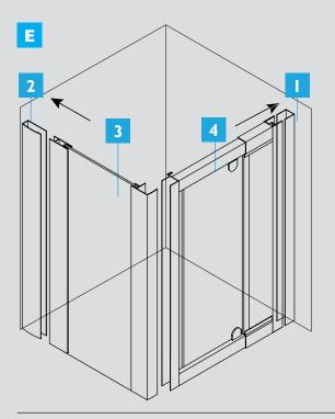
E Slide fixed panel (3) and door front assembly (4) into jambs (1 & 2)
