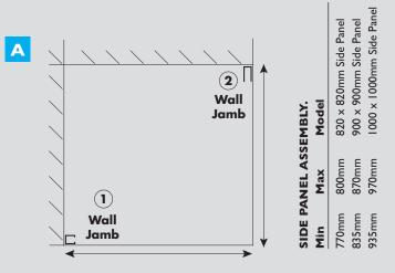
Measure your shower base / shower area. The measurement to the outside edge of the wall jambs (1 & 2) should be somewhere within the minimum and maximum of the screen size. See chart to the left.
