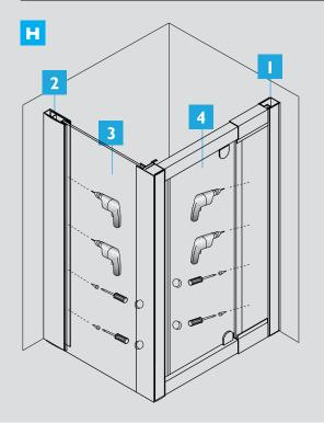
Now drill 4 equally spaced 3.2mm holes into the wall jambs (1 & 2) on the **INSIDE** of the screen. Make sure that your drill holes are more than 20mm back from the glass edge, when using smallest screen size, otherwise you may break the glass.
