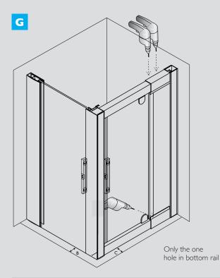
Adjust front assembly and fixed side panel so B=C.This is done by sliding the fixed panel in or out of the wall extrusion for the fixed side. For the front, the top and bottom rails of the front assembly slide apart for adjustment.
