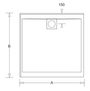
The Flinders New shower base is made from high-strength polymarble compound which is a durable, fully moulded material that is ideal for bathroom applications.
