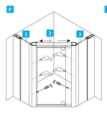
Slide front of fixed panel (2) over extrusion on front door assembly (3). Now drill 4 equally spaced 3.2mm holes on the **INSIDE** of the screen (See aerial view). Fix side panel (2) to front assembly (3) using fixed panel screws 8mm (5). Cap all screws using fixed panel screw caps (6).
