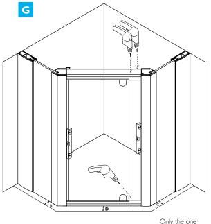
Adjust front assembly and fixed side panel so B=C=D. This is done by sliding the fixed panel in or out of the wall extrusion for the fixed side. For the front, the top and bottom rails of the front assembly slide apart for adjustment.
