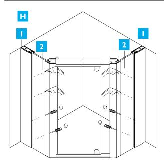
Now drill 4 equally spaced 3.2mm holes into the wall jambs (1) on the **INSIDE** of the screen. Make sure that your drill holes are more than 20mm back from the glass edge, when using smallest screen size, otherwise you may break the glass. Make sure that the holes also go through the aluminium of the
