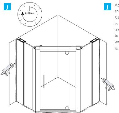
Apply silicone sealer around all external joints of shower screen and allow 24 hours for silicone to set.
