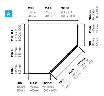
Measure your shower base / shower area. The measurement to the outside edge of the wall jambs (1) should be somewhere within the minimum and maximum of the screen size. See chart to the left.
