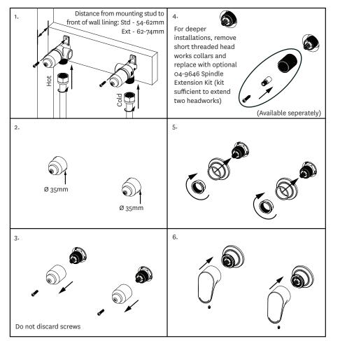
Note: It is the responsibility of the installer to ensure a water proof seal is achieved between the faceplate and the finished surface of the wall. If in any doubt about the quality of the seal, the faceplate should be removed and then reinstalled using silicone to ensure a seal is achieved.
