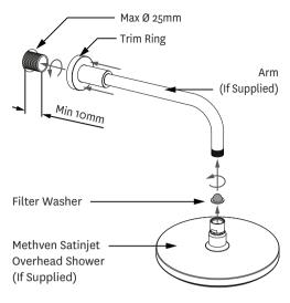
NOTE: Use plumbers tape or similar on ½" male threaded connection to ensure a reliable seal.
